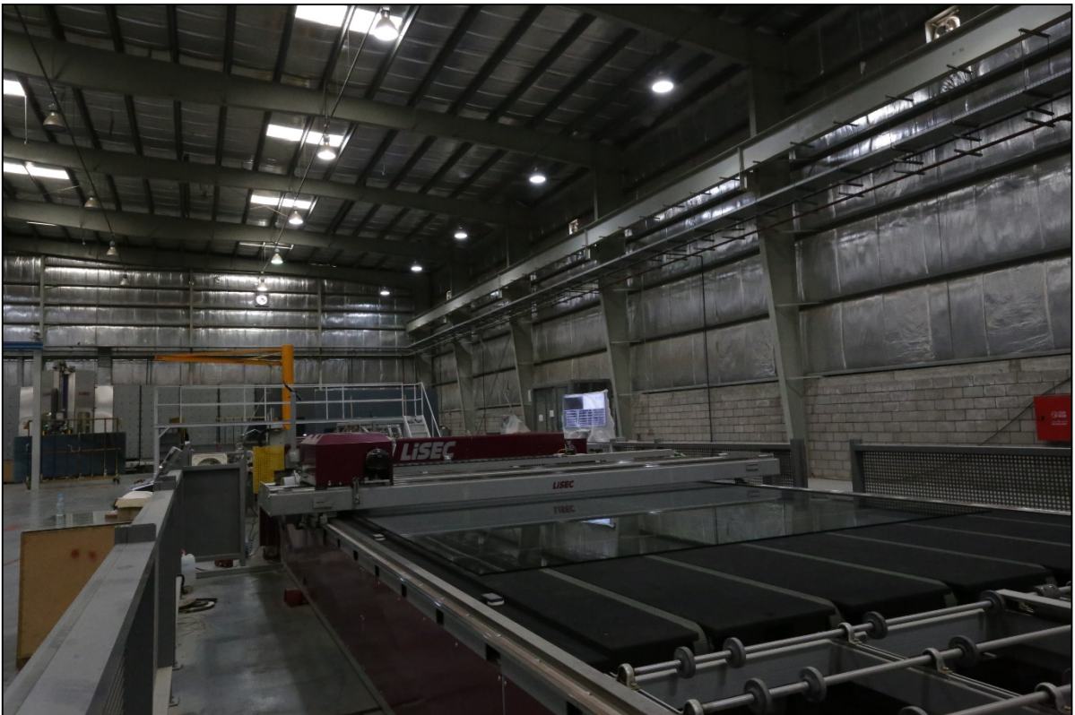
Lisec CNC Glass cutter-automated cutting system for float glass.
