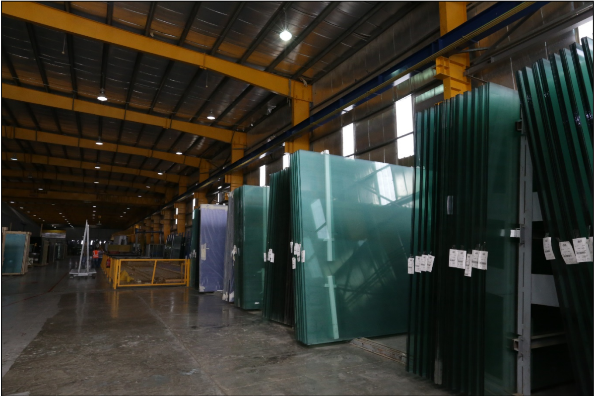
Float glass storage section prior to cut to required dimension.
